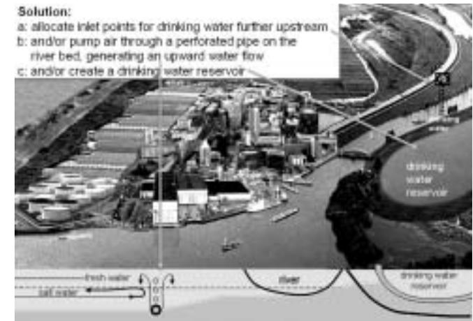
Figure 6: Solutions to avoid salinization of drinking water due to rising sea level
