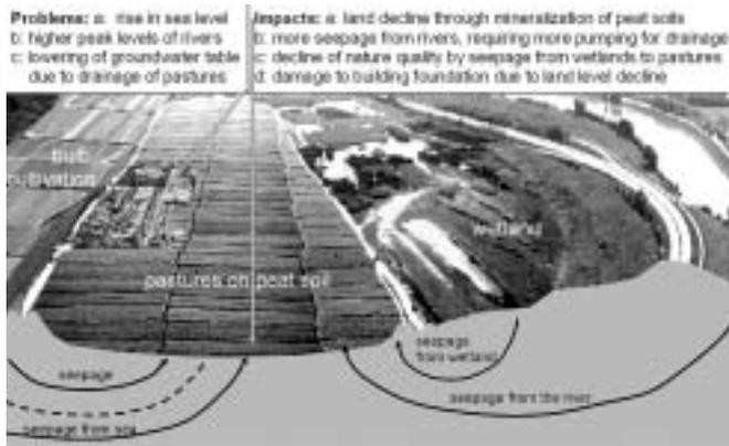
Figure 10: Soil subsidence causing land level decline due to drainage of pastures on peat soil, resulting in high pumping costs, the decline of wetland quality and damage to buildings
