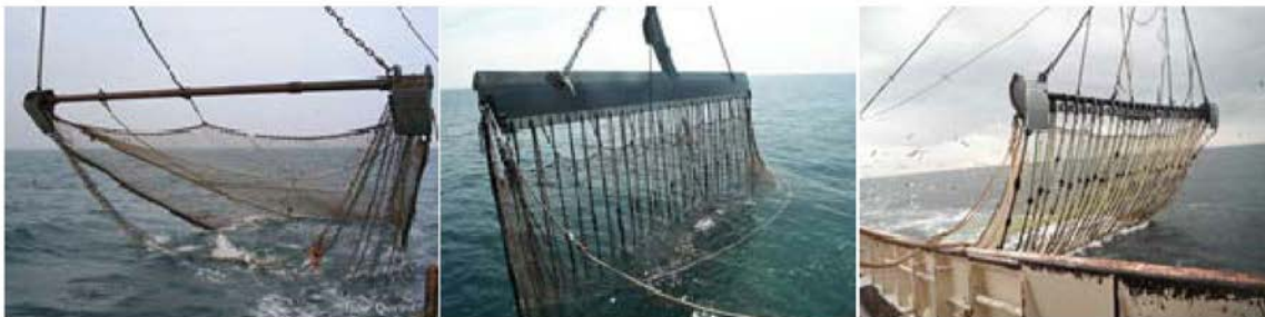
FIGURE 2.1. FROM LEFT TO RIGHT: TRADITIONAL BEAM TRAWL, HFK PULSWING, DELMECO PULSKOR
