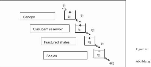
Figure 4: Schematic representation of the reservoir model (HUIJBEN, 2011) Abbildung 4: Schema des Linearspeichermodells (HUIJBEN, 2011)
