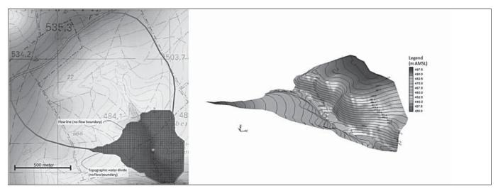
Figure 5: a) Topographical map with elevation, catchment boundary (grey line), model area (black grid) and gravimeter location (green dot), and b) three-dimensional image of the surface level of the modelled area
