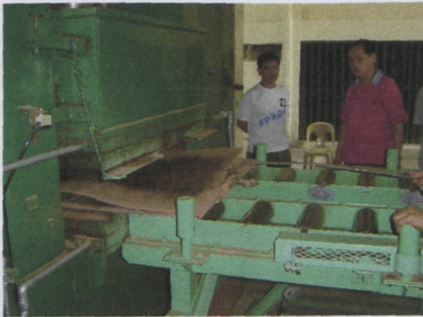
Figure 48 Hot-pressed coir-board leaving the press
