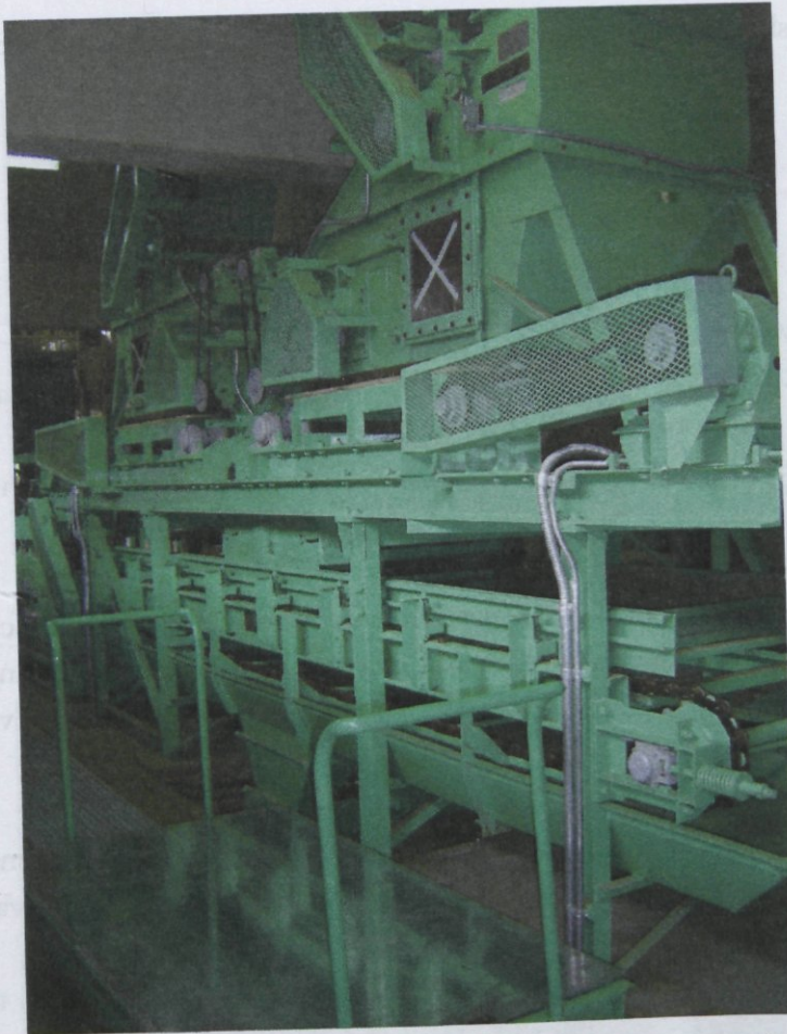
Figure 39 The mat former, showing the mixing section and the transportation section for the carrier sheet
