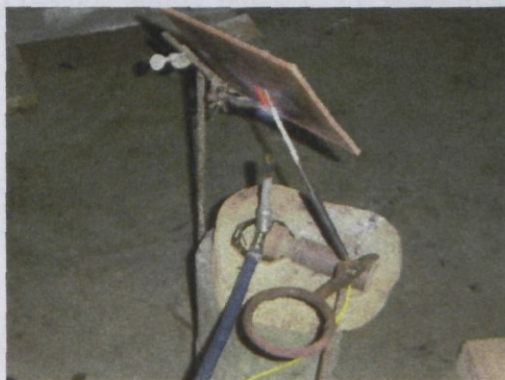
Figure 31 Set-up of fire resistance test at FPRDI.
