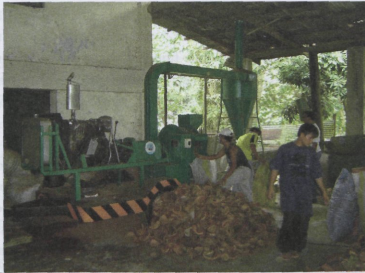
Figure 33 The milling device in operation
