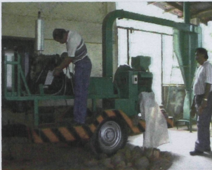
Figure 27 Pilot cutting mill, specially designed for milling coconut husk for application in panel boards.
