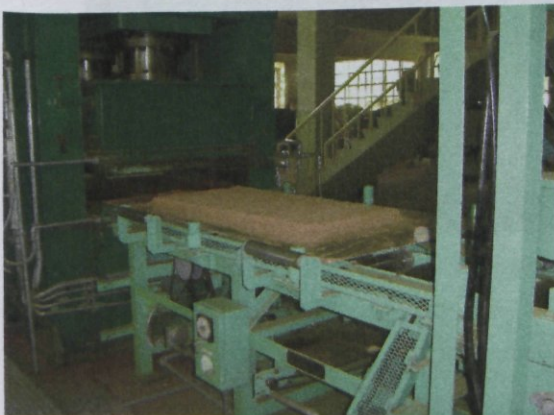
Figure 41 Introduction of the mat in the press
