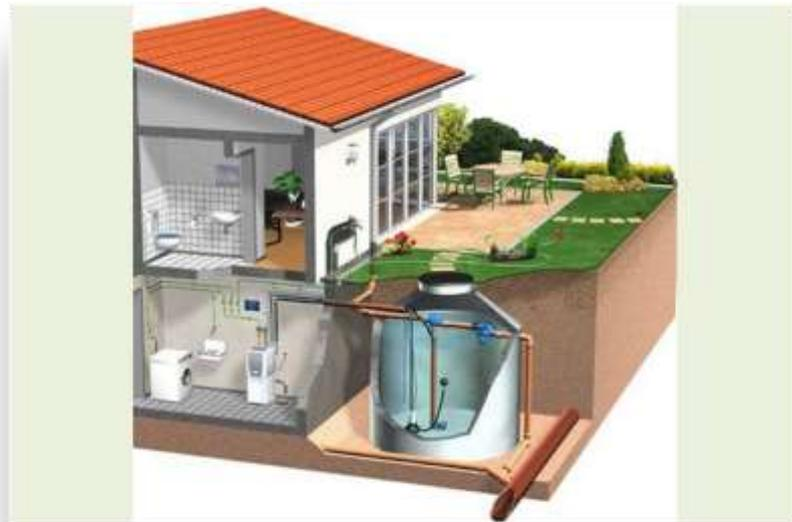
Figure 9: Example of a small scale individual RWH system.
