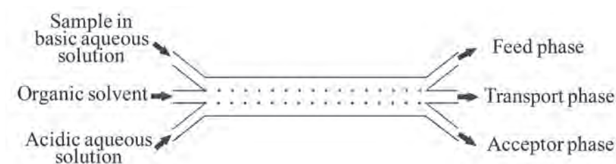
Fig. 1. Schematic representation of the 3-phase chip. Channel dimensions: 100 \mu\text{m} width, 40 \mu\text{m} depth, 3.56 cm length (for each channel).
