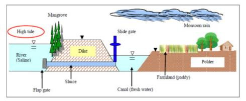
Figure 8 Functioning of a polder in the lower delta (JICA, 2011)
