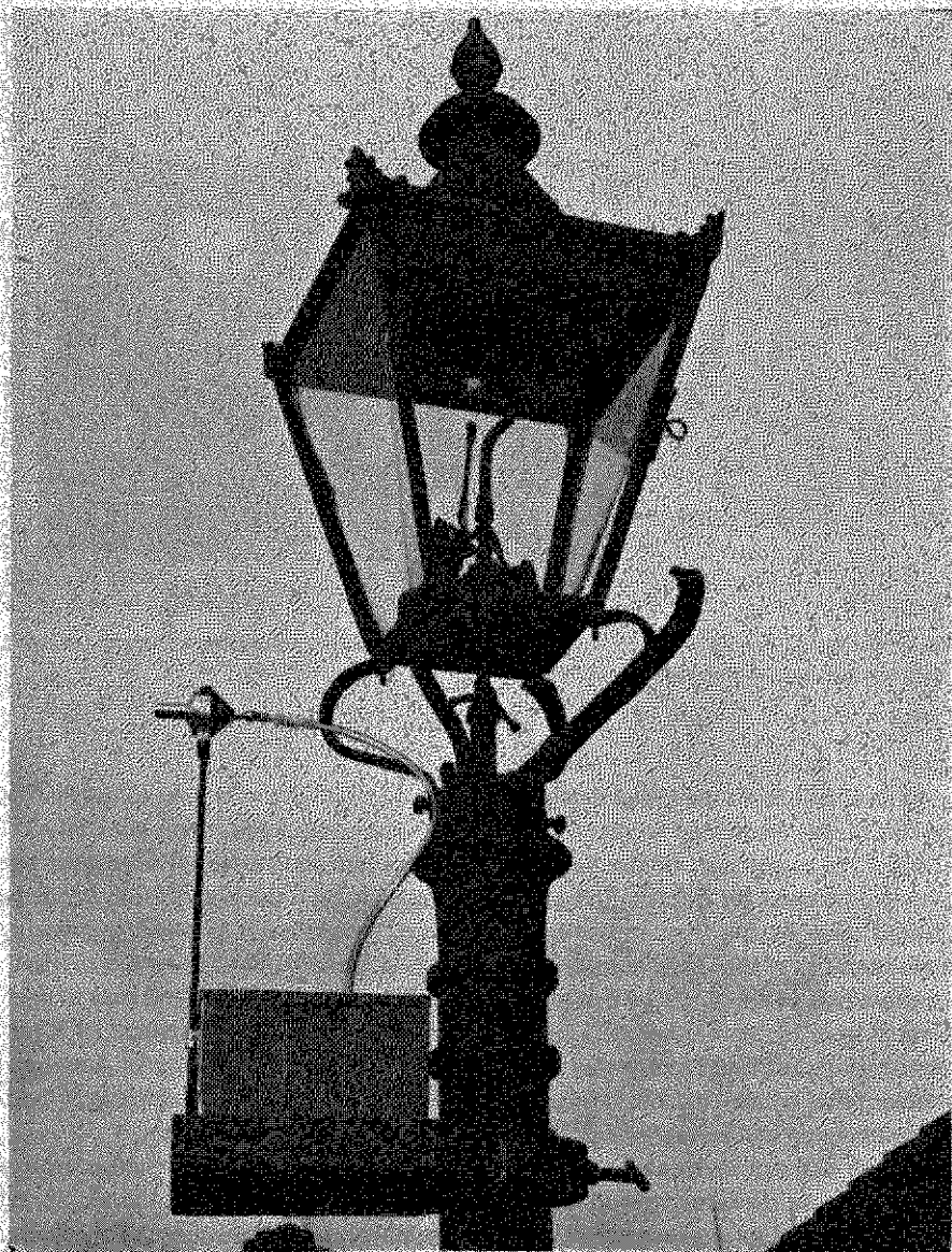
Fig. 7. A portable sampler operated by a 6-volt battery and incorporating time switches to enable sampling to take place over a predetermined period at a number of sites. They can be placed on trays such as the one illustrated, attached to any convenient posts.
