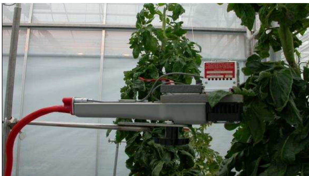
Figure 10. Picture of ADC LCPro+ leaf chamber while measuring leaves of tomato plant.
