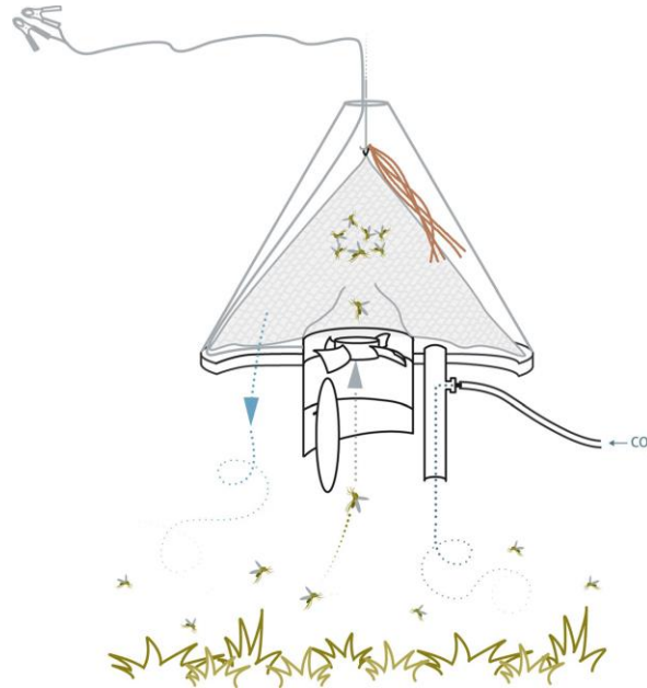
Fig. 8 – Cross-sectional drawing of the Suna trap (Hiscox, Otieno, et al., 2014)
