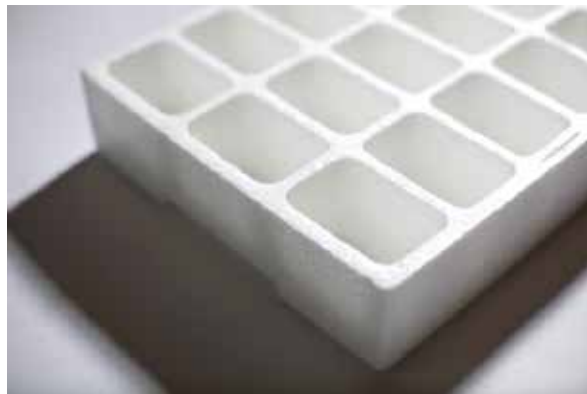
Figure 18. Biofoam ® looks like traditional 'styrofoam', but is made of PLA.
