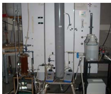
Figure 7.1 The Photographs of the column set: (A). A full view of set-up (B) A closer view with short column filled with Aquamandix (C) short column filled with IOCS.
