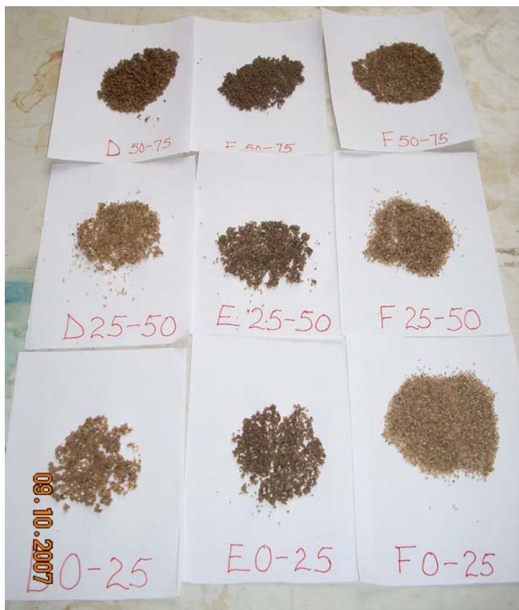
Figure 5.9 A photograph of the manganese coated sand grains taken from the various segments of the filters A, B and C. The samples D0 – 25, D25 – 50 and D50 – 75 represent samples taken from the lowest, middle and top segments respectively of Filter A. Likewise, E0 – 25, E25 – 50 and E50 – 75 represent sand grains from lowest, middle and top segment of Filter B. The F samples come from the Filter C.
