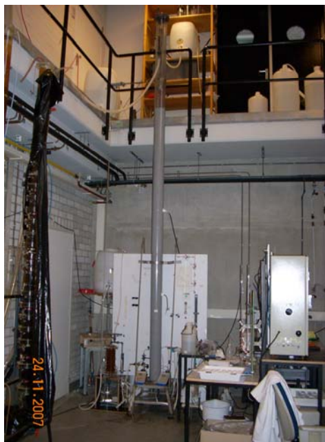
Figure 7.1 The Photographs of the column set: (A). A full view of set-up (B) A closer view with short column filled with Aquamandix (C) short column filled with IOCS.
