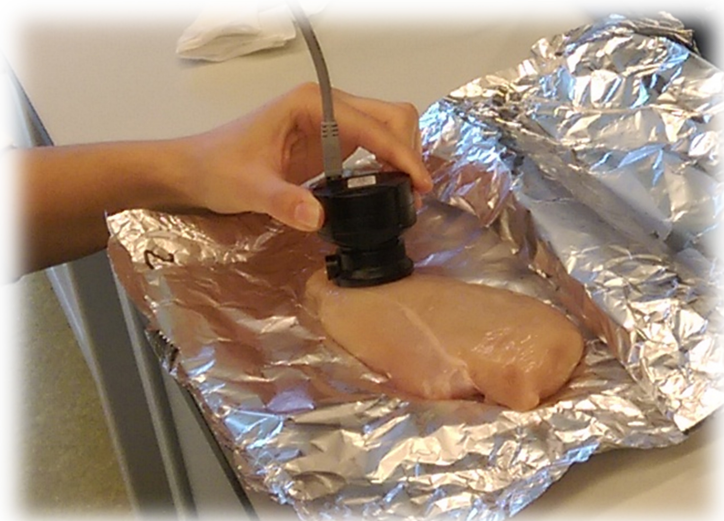
Figure 1. Obtaining NIR spectra of chicken filets with the MicroNIR™ 1700 equipped with rim.
