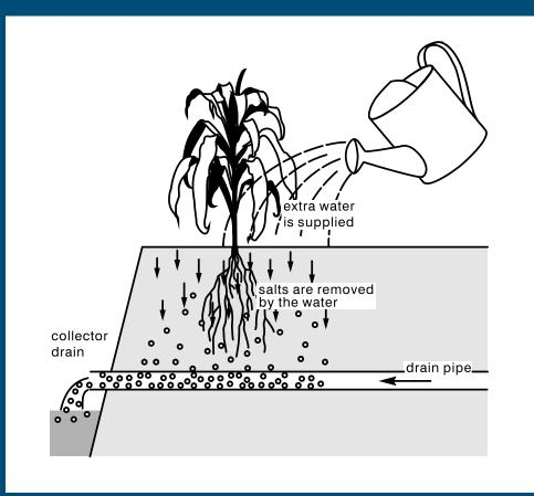
the removal of soluble salts by the passage of water through soil.
