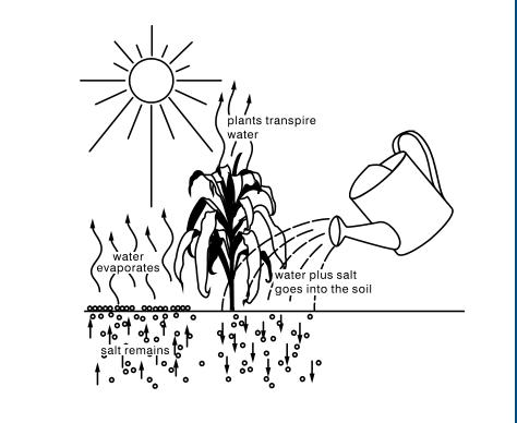
Salinization is the accumulation of soluble salts at the surface, or at some point below the surface of the soil profile, to levels at which they have negative effects on plant growth and/or soils.
