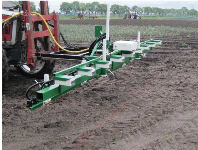
Fig. 2. Leek spraying system consisting of WeedIT sensors in combination with solenoid activated nozzles spraying 0.10\text{ m} \times 0.10\text{ m} targets.
