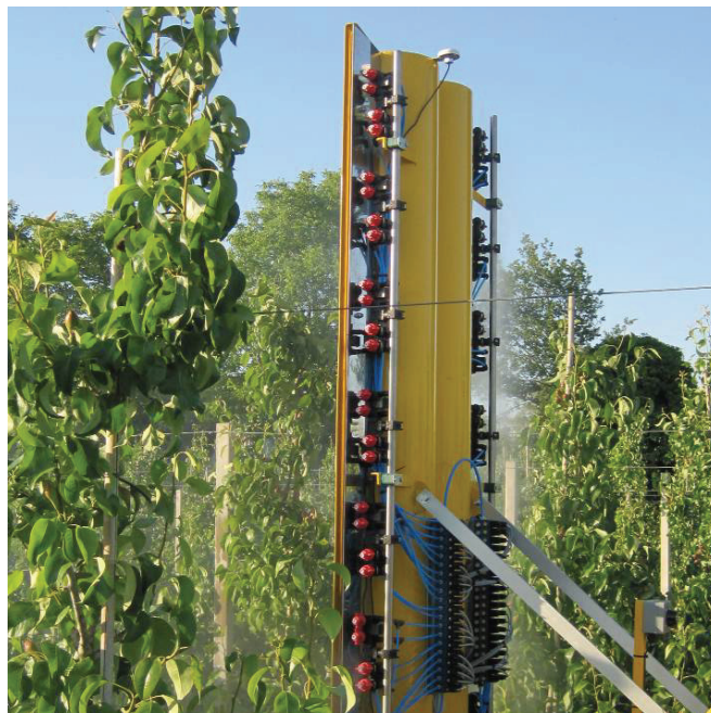
Fig. 3. Canopy Density Spraying system in pear consisting of a laser scanner in combination with Lechler Varioselect pneumatic actuated nozzle bodies.
