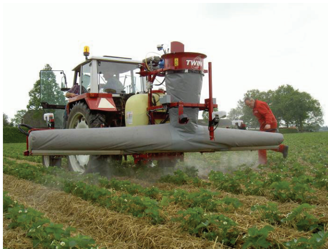
Fig. 1. Strawberry air-assisted spraying system consisting of GreenSeeker sensors in combination with Lechler VarioSelect pneumatic nozzle bodies.
