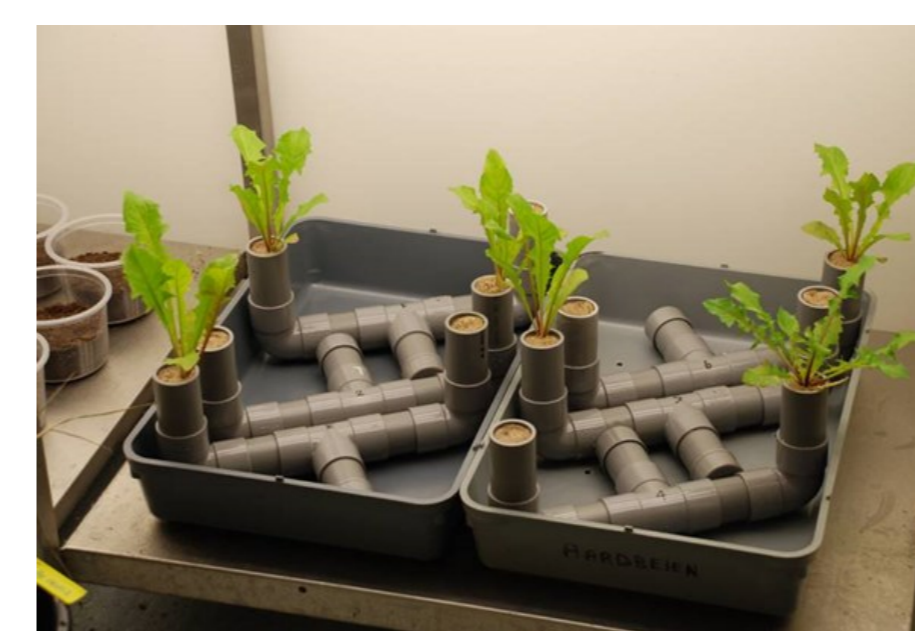
An olfactometer for soil insects. Gauze prevents contact of the grubs with the plant-roots.
