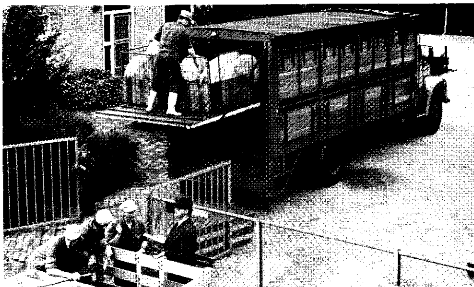
Fig. 10. Loading of the upper deck by the hydraulic lift platform. In the foreground wooden containers with waiting animals.
