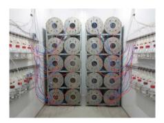
Fig. 1. Experimental CATT system used for eliminating tarsonemids (*Phytonemus pallidus*) or the plant parasitic nematodes *P. penetrans* and *M. hapla* in strawberry runners. Food & Biobased Research, Wageningen UR.
