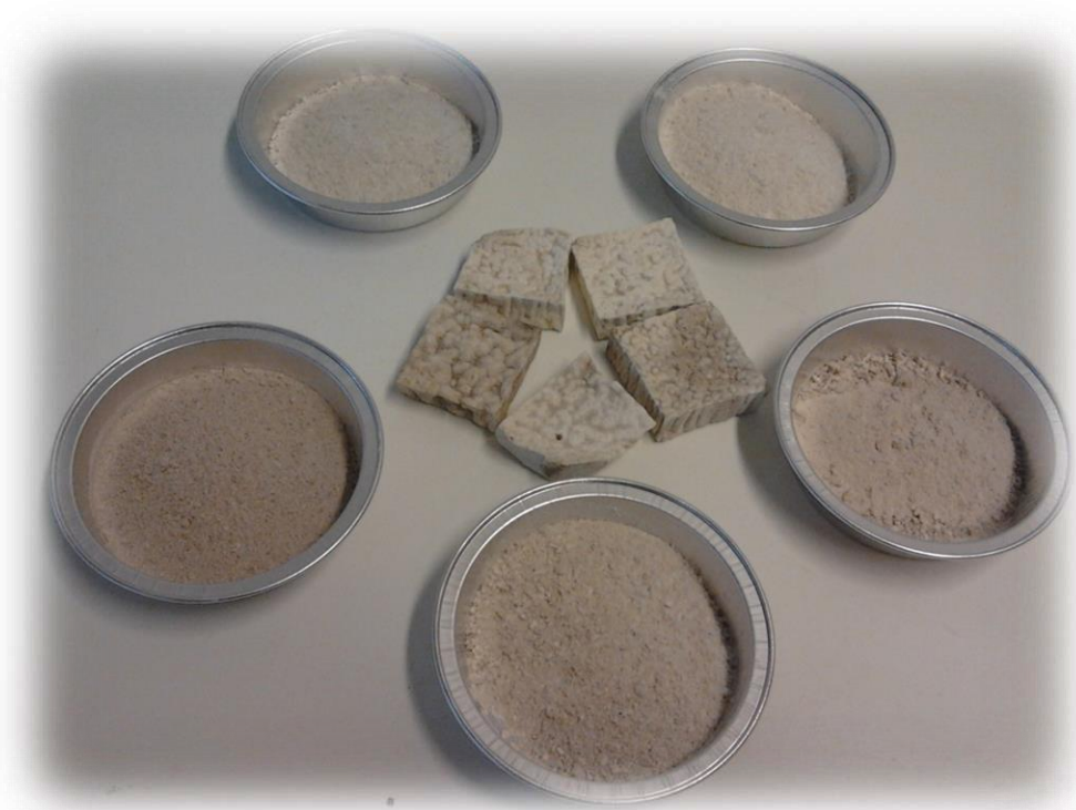
Figure 22: Flour and yam pieces obtained from the drying treatments. Clockwise, starting at the bottom: room temperature, open sun, PoorSolar, OptiSolar2, OptiSolar1.
