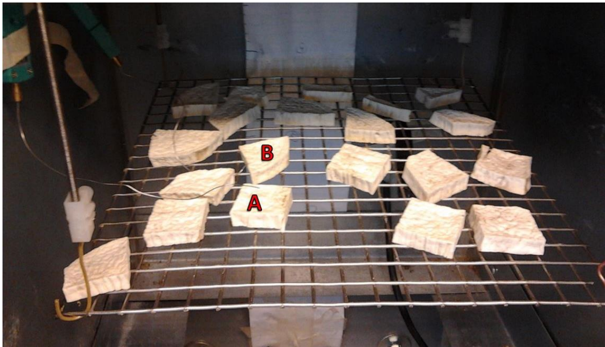
Figure 28: Slices in the drying tray. Sensor A measures air temperature just above the slice (3 mm), sensor B is inserted in the middle of a slice.
