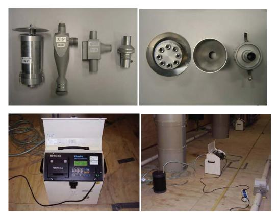
Figure 1 Sampling equipment for PM10 and PM2.5. Photograph upper left (from left to right): inlet, PM10 and PM2.5 cyclone collector and filter holder. Photograph upper right: adapted inlet for cyclone collectors. Photograph left bottom: the constant flow pump. Photograph right bottom: a constant flow pump connected to the condensed water collection vessel
