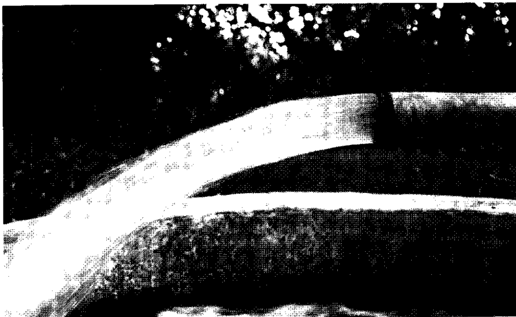
Photo 2. Flow from a horizontal pipe.
