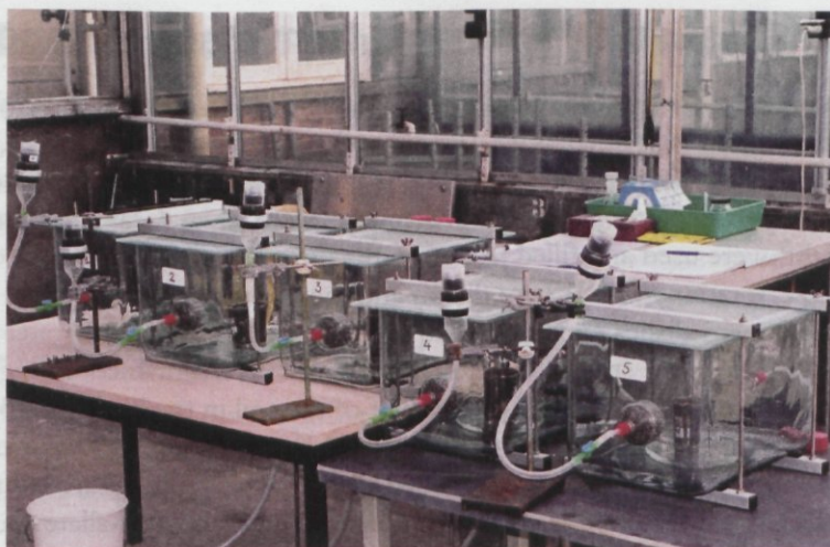
Picture 3. Volatilization measurement from glass beakers filled with soil placed in the compartments.
