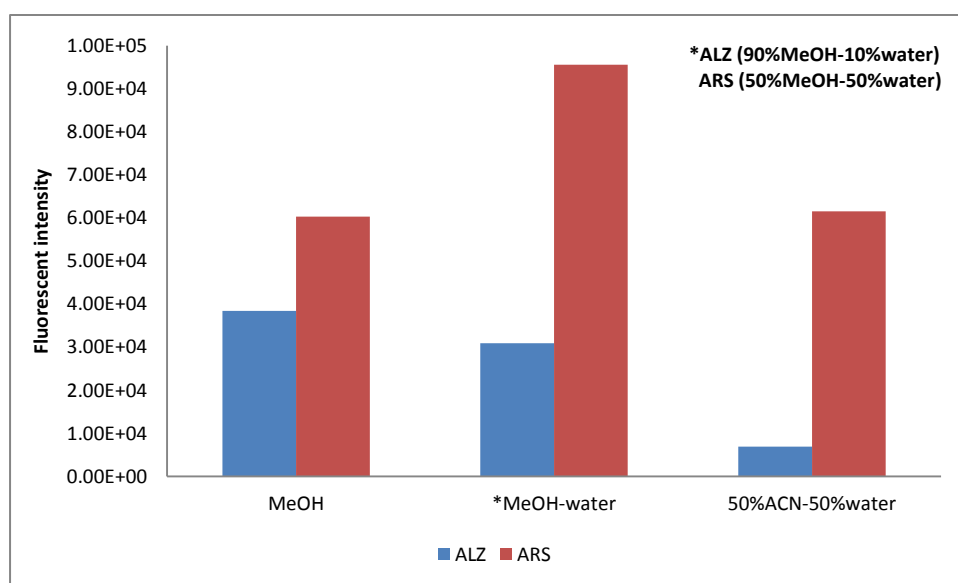
Figure 9. The fluorescent intensity of alizarin (ALZ) and ARS ( \lambda_{Ex} 469nm; \lambda_{Em} 610nm)
