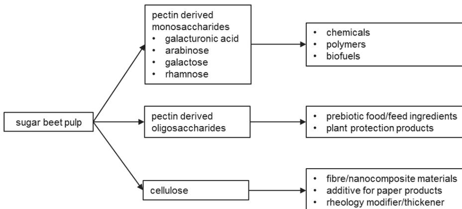
**Figure 6.2.** Biorefinery cascade of sugar beet pulp: simultaneous production of different value-added biobased products.
