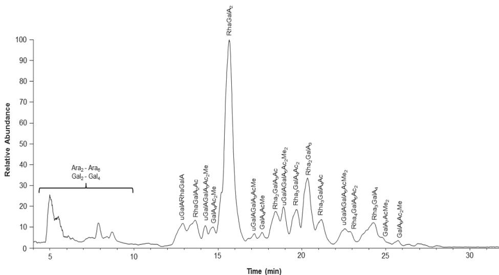
**Figure 4.1.** Hydrophilic interaction chromatography (HILIC) elution pattern of sugar beet pectic oligosaccharides (SBPOS). Peak annotation: Ara, arabinose; Gal, galactose; GalA, galacturonic acid; uGalA, unsaturated galacturonic acid; Rha, rhamnose; Ac, acetyl group; Me, methyl ester.
