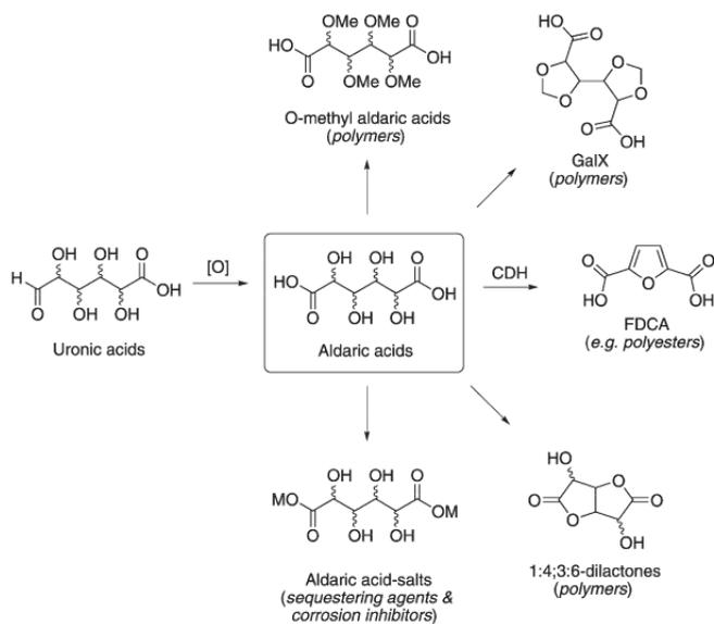
**Figure 1.6.** Route from uronic acids to aldaric acids, derived products and main applications. Legend:  $[O]$ , oxidation;  $CDH$ , cyclodehydration [83].
