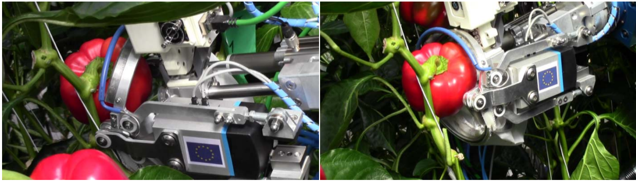
Figure 7-12. Comparison of a grasp pose calculated when stem localization was disabled (left) and enabled (right). Due to the non-ideal pose in the left figure, the end-effector pushed against the stem and did not grasp the fruit. In the right figure, the end-effector successfully grasped and cut the fruit.
