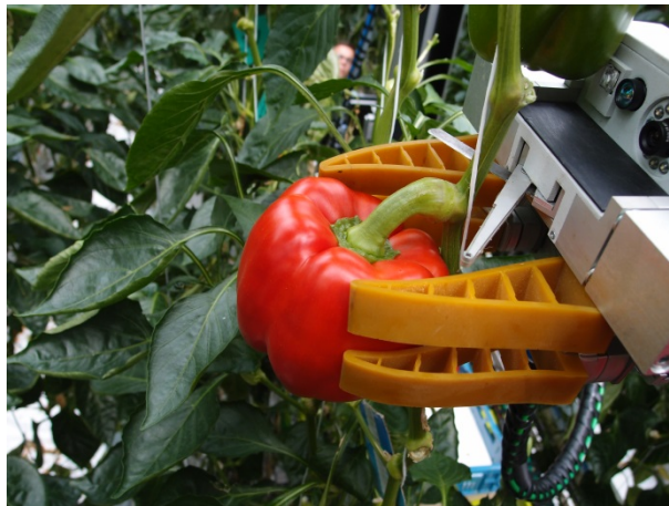
Figure 7-9. Photo of a grasp pose calculated for a target fruit when stem detection was disabled. Upon cutting, the mechanism would damage the stem present between the scissors.
