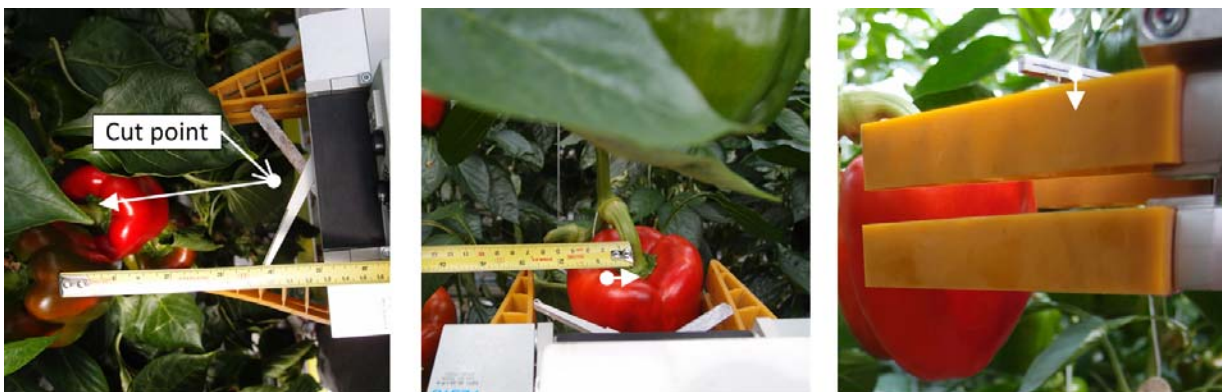
Figure 7-7. Measuring the positioning error of the end-effector in depth (left), width (centre) and height (right). White arrows indicate the error measured with respect to the cut point defined between the scissors.
