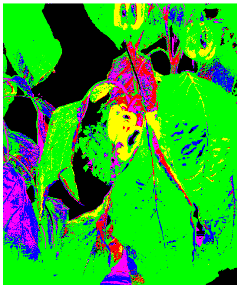
Figure 4-4. Classification of vegetation into five classes: stem (red), top of a leaf (green), bottom of a leaf (blue), fruit (yellow) and petiole (magenta). Black parts are either background regions or overexposed regions.
