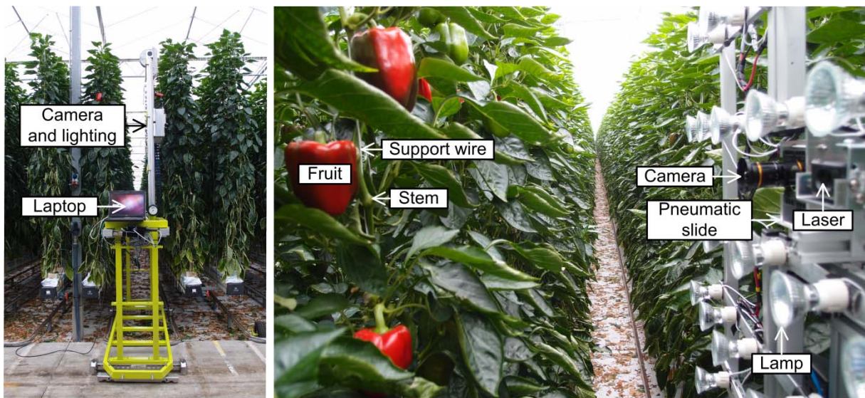
Figure 5-1. Experimental set-up comprising a cart with a height-adjustable imaging set-up on top (left). Detailed view of the imaging set-up during recording in a row (right).
