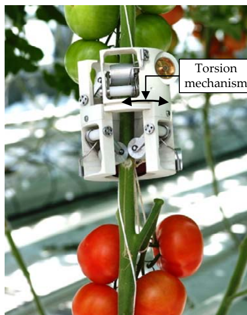
Figure 2-15. Functional model of a climbing robot for tomato. The torsion ability of the frame allows for peduncle or leaf avoidance during movement along the stem. Photograph courtesy of Bart van Tuijl, Wageningen UR
