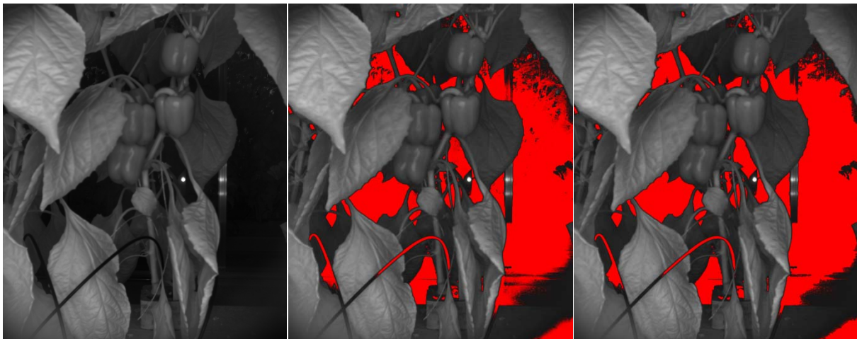
Figure 3-6. The background of the image (left) was segmented (centre) from other objects in the scene using a gray value threshold ( \leq 27 ). Subsequently holes were filled (right). Unfortunately, part of the dripper is classified as background whereas it should have been classified as a hard obstacle.
