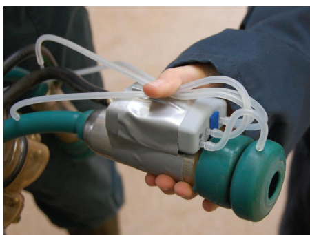
silicon tubes connect straws to VaDia
