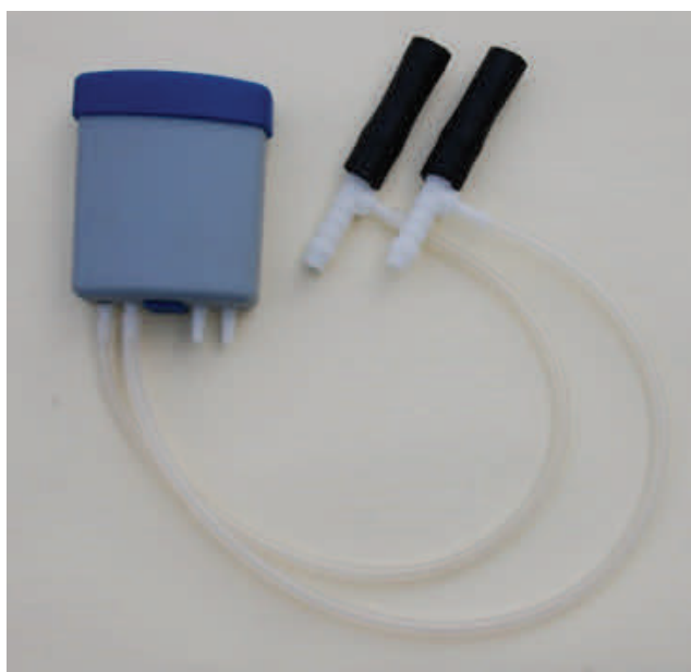
VaDia for pulsator test (T-pieces supplied in VaDia kit)
