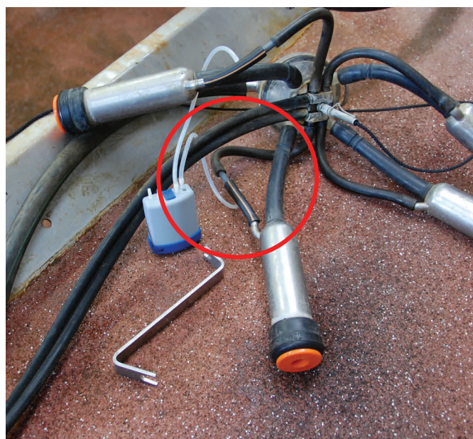
VaDia connected to milking cluster for pulsator dry-test
