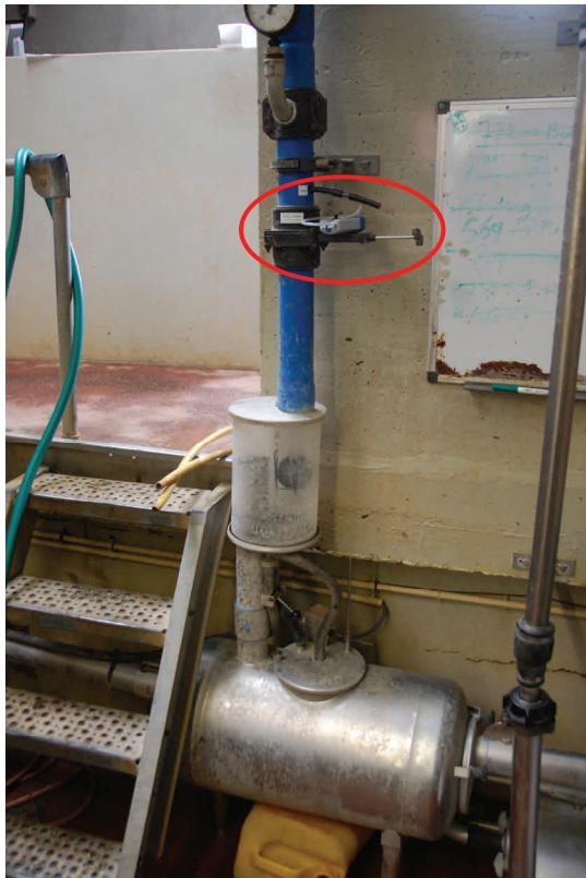
VaDia connected to the milk receiver at point Vm (test point may vary due to local legislation)
