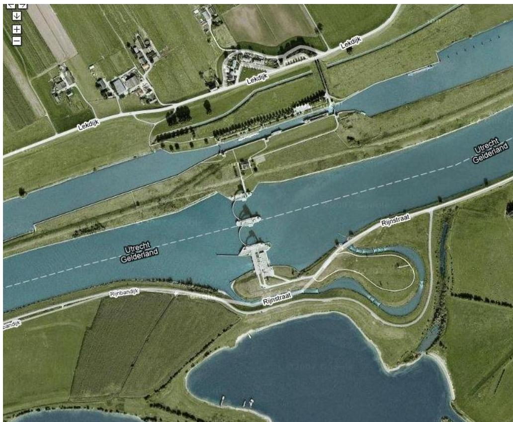
In order to give passage to the navigation in these short periods (some weeks per year) of nearly closed weirs, these weirs are mostly combined with one or two navigation locks. Although with some delay in the order of 15 - 30 minutes per passage, these locks make it possible to overcome the created differences in heads, here estimated as about 5 meter.
