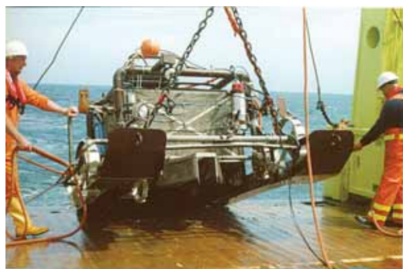
Figure 3. Triple-D dredge for sampling larger sized and lower abundant infauna and epifauna. Sampling area: a strip 80 m long and 20 cm wide (16 m 2 ) to a depth of 18 cm. Meshsize of the netting 1.4 cm stretched (Bergman and van Santbrink, 1994).
