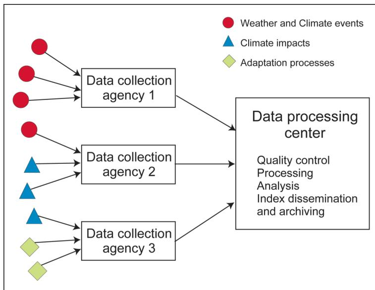
Proposed structure and process of monitoring climate change, impact, and adaptation parameters, and for translating them into indicators for New York City
