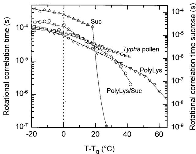
FIGURE 4 Rotational correlation time ( $\tau_R$ , s) of CP in the cytoplasm of *Typha latifolia* pollen (*squares*), and in sucrose (*triangles*), PolyLys (*inverted triangles*) and a 1:1 (w/w) mixture of PolyLys and sucrose (*circles*) as a function of  $T - T_g$ . Dashed line indicates  $T_g$ . All samples were equilibrated to 33% RH, except for sucrose and the mixture of PolyLys and sucrose (3% RH).
