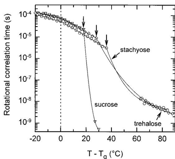
FIGURE 1 Rotational correlation time ( $\tau_R$ , s) of CP in different sugars as a function of  $T - T_g$ . Dashed line,  $T_g$ ; arrows, the critical temperature  $T_c$ ; inverted triangles, sucrose equilibrated to 3% RH; diamonds, trehalose equilibrated to 33% RH; circles, stachyose equilibrated to 33% RH.
