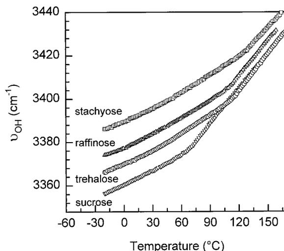
FIGURE 3 The wavenumber of the OH stretching vibration ( $\nu_{\text{OH}}$ ,  $\text{cm}^{-1}$ ) for different sugars as a function of temperature. Sugar glasses were first heated to remove residual water. Inverted triangles, sucrose; circles, trehalose; triangles, raffinose; squares, stachyose.
