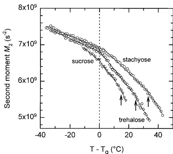
FIGURE 2 The second moment ( $M_2$ ,  $\text{s}^{-2}$ ) of immobile protons of different sugars as a function of  $T - T_g$ . Dashed line,  $T_g$ ; arrows, the critical temperature; inverted triangles, sucrose equilibrated to 3% RH; diamonds, trehalose equilibrated to 33% RH; circles, stachyose equilibrated to 33% RH.
