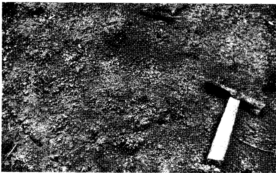
Photo 1 Belterra clay exposed at the surface. After exposure to the weather, the very heavy, kaolinitic clay, termed Belterra clay, falls apart into very fine blocky elements that are very resistant to destruction
