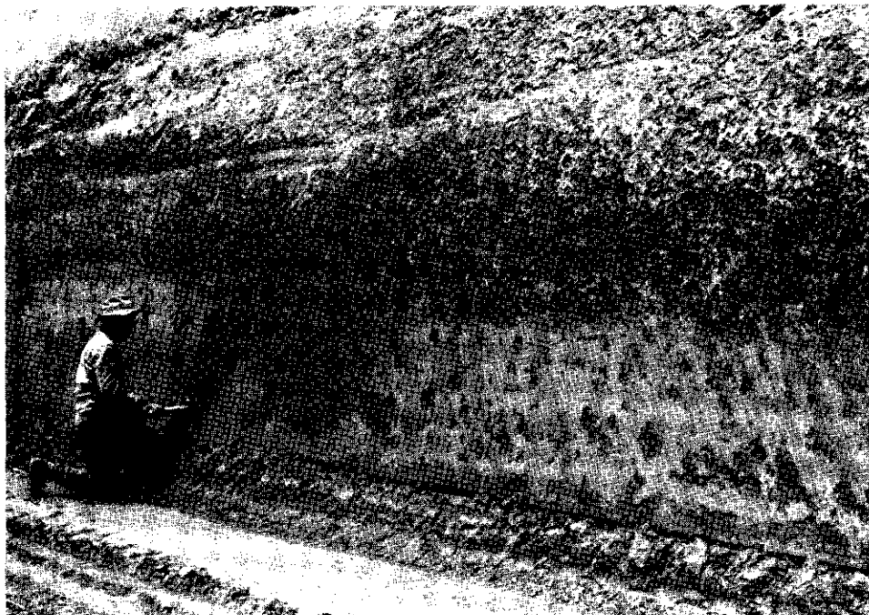
Photo 4 Ligação type of concretions capping unmottled, friable earth. The absence of any soft plinthite, the sharp and irregular lower boundary of the layer of hard plinthite, the subrounded form of the concretionary elements themselves, and the absence of any arrangement of these elements, together indicate that the layer of hard plinthite was not formed in situ, but is of alluvial origin (BR-14, km 370 ca.)
