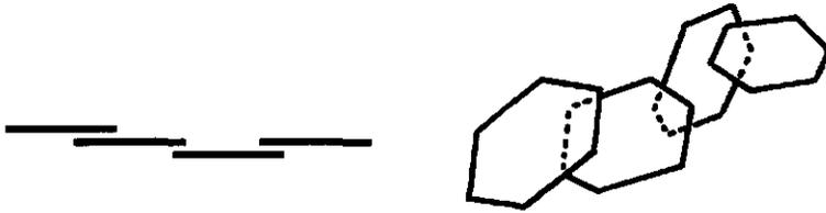
Fig. 61. Chain type flocculation of calcium bentonite at low salt concentration
