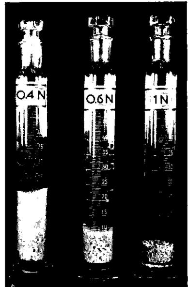
FIGURE 4. The swelling of Na-bentonite in dependence of salt concentration. 1 g granules in, from left to right 0.4 N, 0.6 N and 1 N solution
