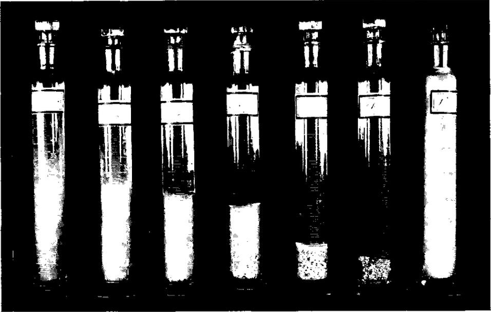
FIGURE 3. The swelling of Na-bentonite in dependence of salt concentration. 1 g granules in, from left to right 0.002 N, 0.02 N, 0.2 N, 0.4 N, 0.6 N, 1 N, and 1 N swollen in distilled water, salt added afterwards.
