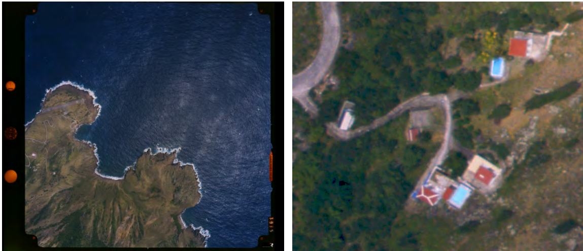
Figure 4 Example of an aerial photograph for Saba from 11 April 1991 with a flight scale of 1:8000 and a spatial detail of approximately 20 cm. Left Figure shows entire aerial photograph and right Figure a detail of the same photograph (copyright by Dotka Data BV – ARCADIS).
