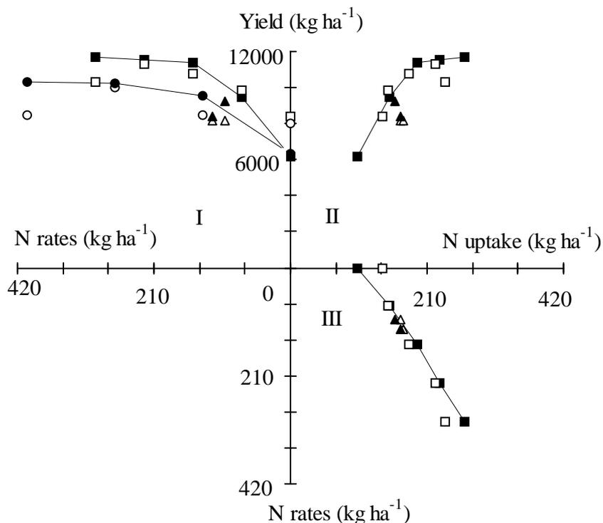
Figure 4.3 Three-quadrant diagram of measured (for SE see Table 4.2) and simulated yield, N uptake, and applied fertilizer N. Simulated (●) and measured (○) values for experiment I with 0, 135, 270, 405 kg N ha<sup>-1</sup> in 2001; simulated (■) and measured (□) values for experiment I with 0, 75, 150, 225, 300 kg N ha<sup>-1</sup> in 2002; simulated (▲) and measured (△) values for experiment II in both 2001 and 2002.
