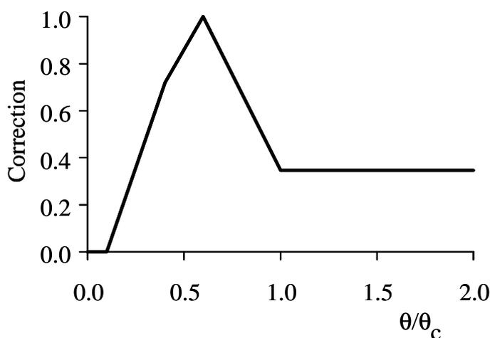
Figure 6.4 Multiplication factor for relative rate of decomposition of organic matter as a function of relative soil moisture content.  $\theta$  is actual soil water content and  $\theta_c$  is soil water content at field capacity, both in the same units.
