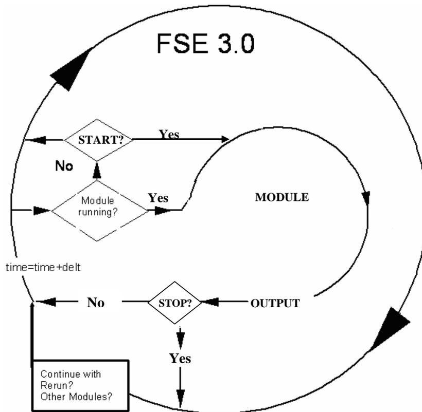
Figure 6.1 Structure of the FSE3.0 (Fortran Simulation Environment) shell to drive modules.
