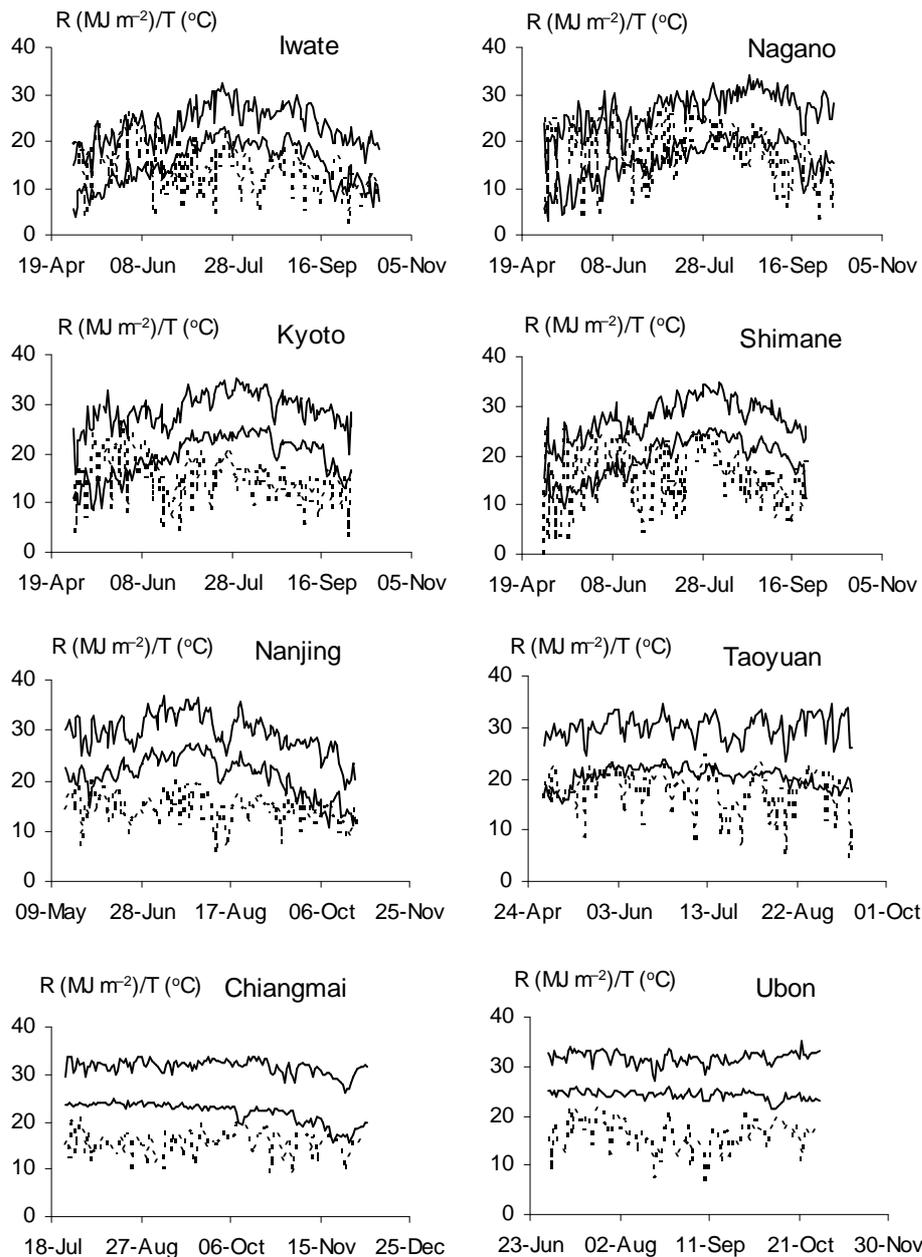
Figure 3.1 Average solar radiation ( $R$ ) and temperature ( $T$ ) of two years during rice growth at eight locations in Asia. Solid lines are maximum  $T$  and minimum  $T$ , dotted lines are solar radiation.
