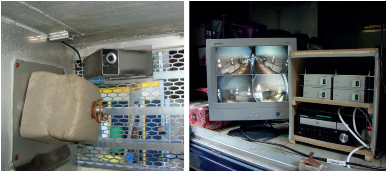
Figure 2.9 Video camera positioned in the upper corner of four of the five compartments per vehicle. Recording devices were placed in the front of the vehicle to monitor whether or not recording was activated
