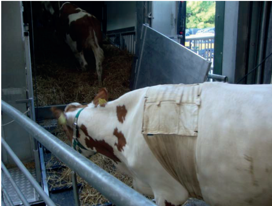
Figure 2.6 Data loggers housed in a stainless steel container and secured in a pouch on the back of the animal to register ECG continuously
