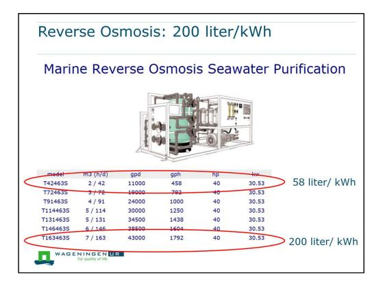
A reverse osmosis device shows to provide some 200 liters of fresh water from a kWh of electricity
