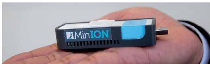
New technologies develop rapidly, the picture shows a portable $900 disposable Oxford Nanopore sequencer, with USB support.
