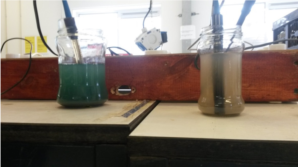
Figure 17: The pH and RedOx meter solution on the left turned blue while the EC meter solution on the right didn't change.
