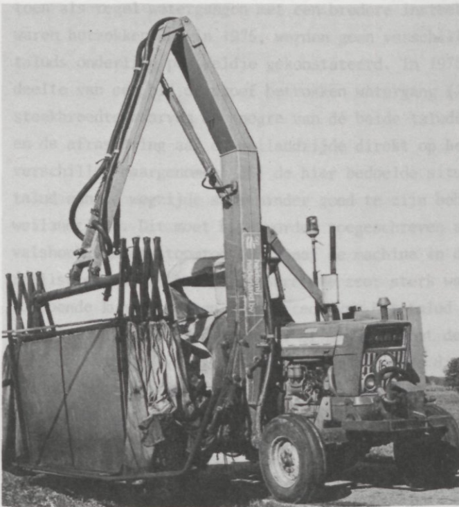
Fig. 6. Steam distributor in transport position. The operating tractor with hydraulic lift equipment coupled behind the steaming machine.
