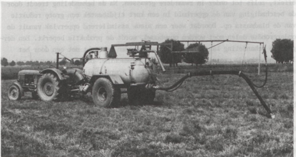
Fig. 1. Tank adapted for the supply of water and soil. Similar tanks, without special adaptations, are used on farms.
