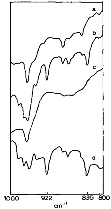
Figure 48a, b, c, d. Infrared spectra of beef tallow. a. Solid beef tallow, \alpha form; 20^{\circ}\text{C} b. Solid beef tallow, \beta' form; 14^{\circ}\text{C} c. Liquid beef tallow; 55^{\circ}\text{C} d. Solid beef tallow, \beta' form; 14^{\circ}\text{C} , compensated with beef tallow in the liquid state; 55^{\circ}\text{C}
