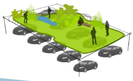
The tramlines green strategy is recommended to implement during the reparation and maintenance period of tramlines, which happens once in a while. By replacing the paving material (normally concrete tiles) underneath the tramlines by vegetation, the green spaces of the city will increase. Additionally, it creates a safer cycling and walking environment for cyclers and pedestrians since the green tramlines also function as a separation line between tramlines and cycle-pedestrian pavements.
