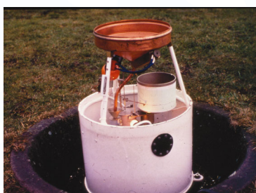
Figure 1. Example of a self-recording rain gauge (without lid).
