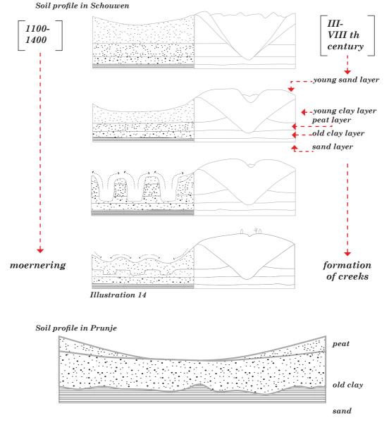
Picture 14. The process of 'moernering': digging out the peat and the final ondulating landform.
