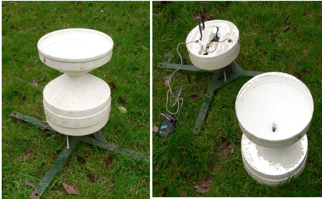
Figure 6: Tipping bucket rain gauge in closed and open position.
