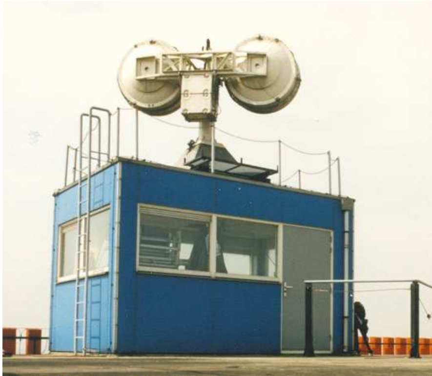
Figure 2: The X-band weather surveillance radar, SOLIDAR, which was operated by Delft University of Technology.
