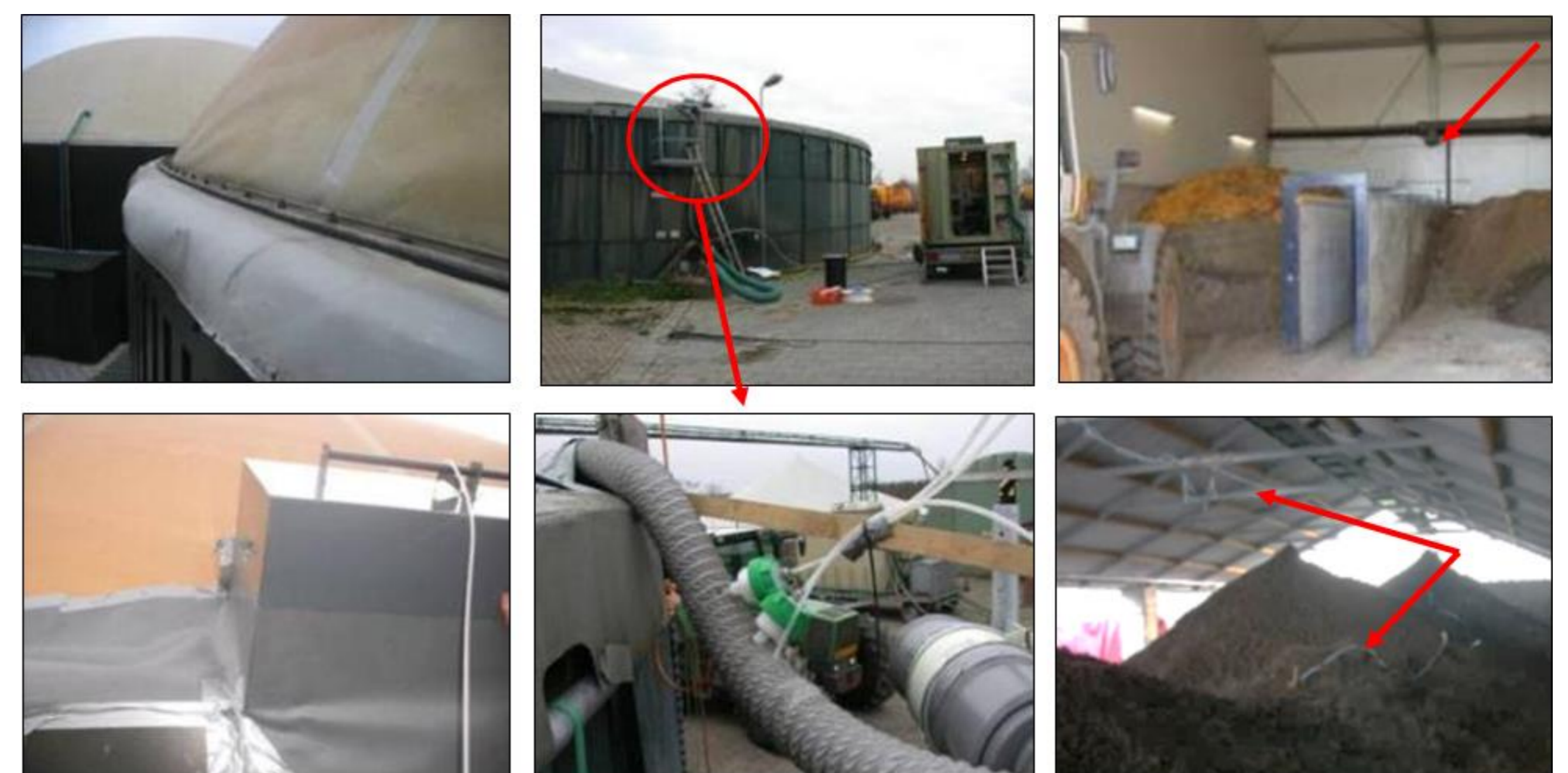
Figure 2. Example of different emission sources and measurement equipment at a manure treatment installation [2].
