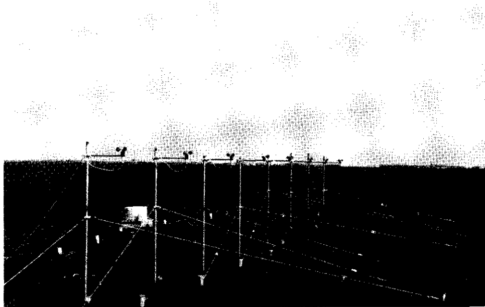
Photo 4. Relative calibration of cup-anemometers in the field.
