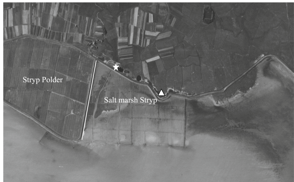
Fig. 3 Pattern of ditches and wooden groynes constructed to enhance sedimentation and reclamation of new agricultural land on the east side of Stryp Polder (where also the patterns of the old reclamation works are still visible, as well as the historical dike), viewed on an aerial photograph taken by the Royal Air Force (UK) on 4 August 1944 (source: Land Registry Office or 'Kadaster'). The pumping station is marked by a white star. A white line indicates a stretch of dike that was outwardly extended in the 1960s; a stretch that is straightened later, is marked by a white triangle
