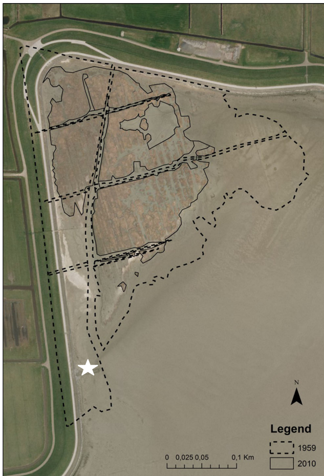
Fig. 6 Salt-marsh area in 1959 (dashed line) and 2010 (solid line) (source: Kadaster). The star marks the groyne placed in 2010 to prevent erosion of the dike by the gully
