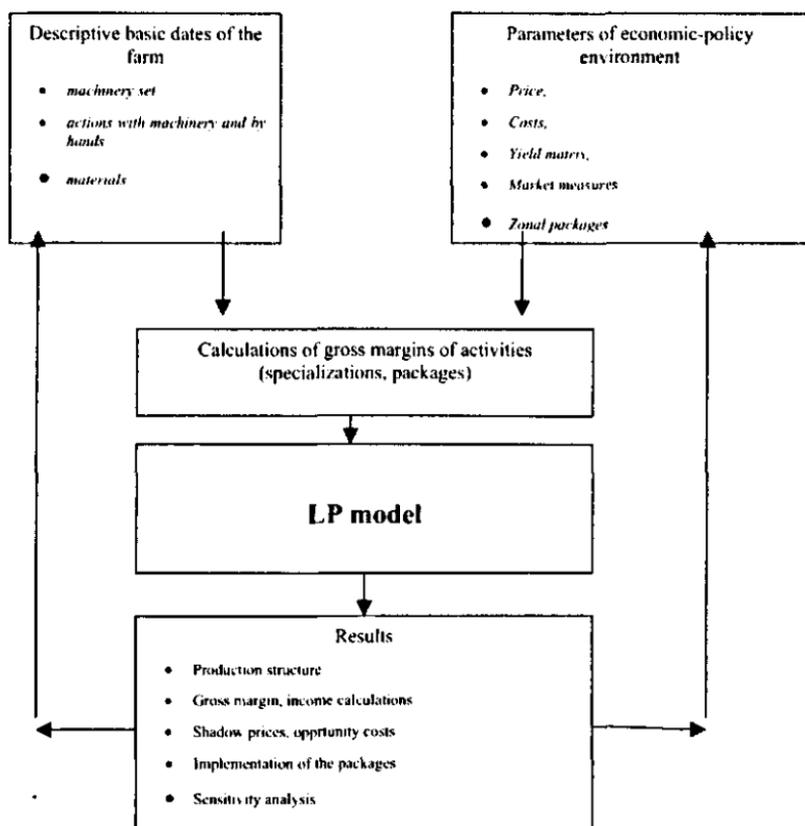
Linear programming presents a collection of relevant technical opportunities by separate activities in a matrix. The rows of the matrix form the constraints that represent the technical relation between the activities. Given the objective function, the solution procedure determines the optimum solution considering all activities and restrictions simultaneously. New production techniques and packages can easily be incorporated by means of adding new activities to the model.
