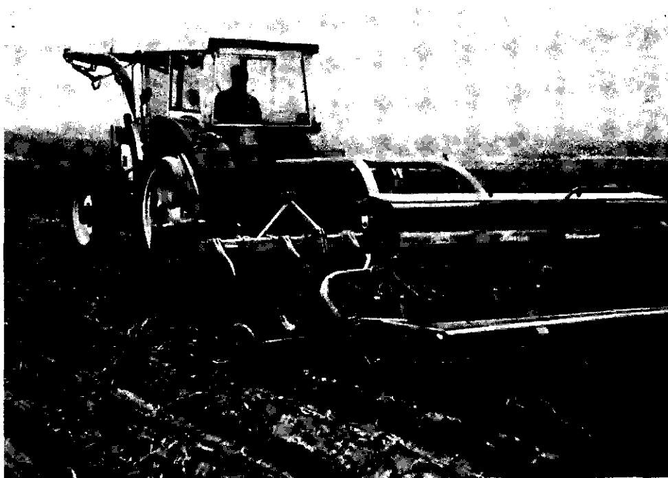
Fig. 4 Combination of fixed-tine cultivating and drilling of winter wheat in one pass (System C).
