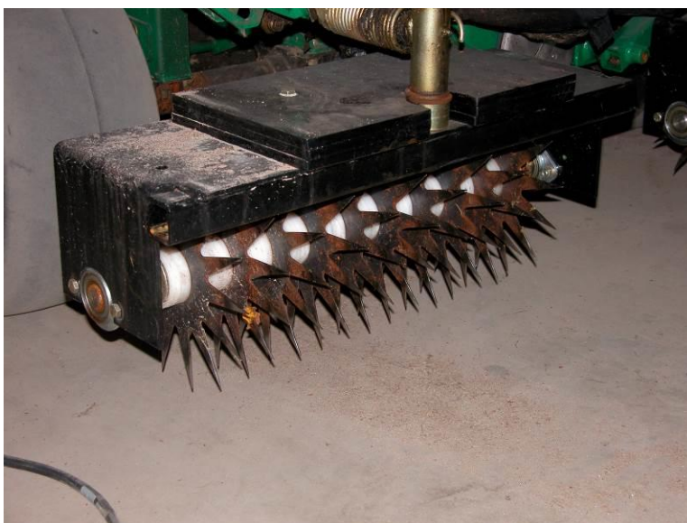
Figure 7-19. Spiking attachments aid with increasing infiltration and can affect significant amounts of surface areas. Source: Frank Rossi.
