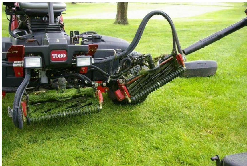
Figure 10-11. Prior to washing equipment, removing clippings while over grass (top) or a pad (bottom) with an air hose or prewash reduces the amount of organic debris in the wash water. Source: Robert Alonzi.
